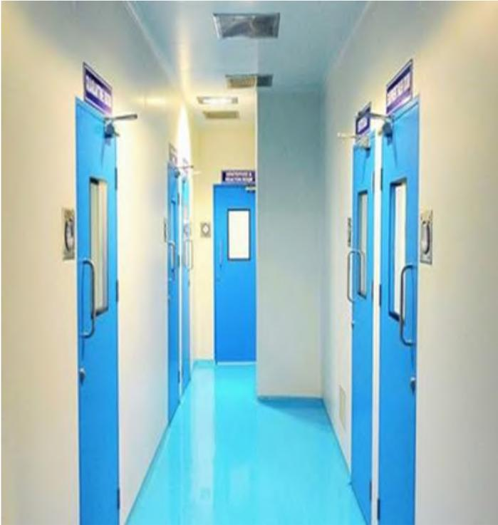
We are the Leading Manufacturer and Supplier of Clean Room Fire Doors. The Cleanroom door is exposed to intense cleaning every day with a variety of strong chemicals to assure high levels of hygiene. Made from Galvanized and Stainless Steel, these flush doors are compact, stable, and strong.
