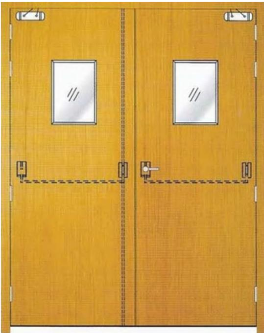
Envirotech are involved in the manufacturing and supply of premium quality wooden fire doors which are installed in buildings to used as part of a passive fire protection system to reduce the spread of fire and smoke between separate compartments.
